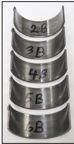
Above left: The rod and main bearings show no sign of "grabbing" from the loss of oil pressure. Above right: Cylinders from Tucker's aircraft still show the "cross-hatch" from honing and no scuffing, something you would not expect to see from a loss of oil pressure.
