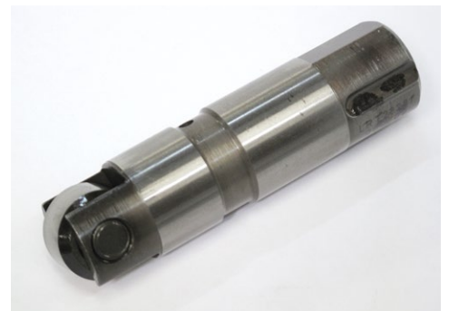
Left: Ly-Con's highly modified engines use roller lifters. The ones removed from Tucker's aircraft had no damage or scarring.
