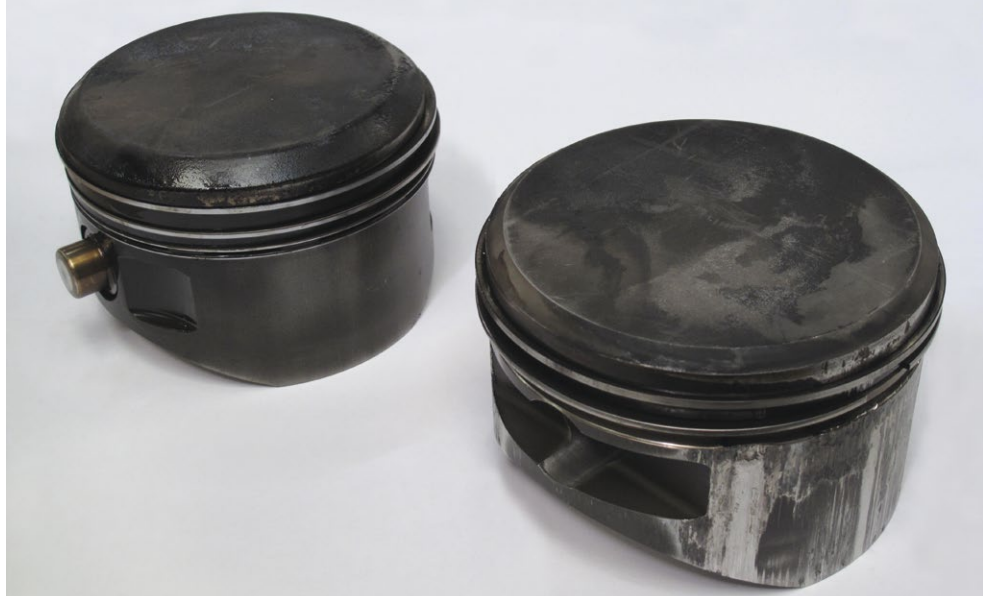
Above: Can you guess which piston was removed from Sean Tucker's aircraft? If you guessed the one of the right, you are incorrect. Surprisingly, the piston on the left is from Tucker's aircraft and sustained no noticeable damage; the piston on the right shows the damage that was expected to occur during his six minute flight with nearly no oil.
