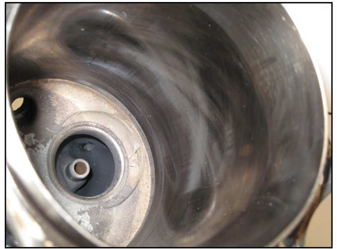
Above left: The rod and main bearings show no sign of "grabbing" from the loss of oil pressure. Above right: Cylinders from Tucker's aircraft still show the "cross-hatch" from honing and no scuffing, something you would not expect to see from a loss of oil pressure.
